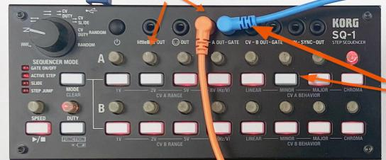
Gate output triggers envelope at each lit step. Adjust pattern by turning steps on/off.
